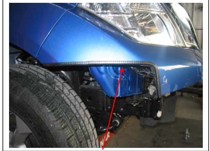
Figure 8: 3mm clip lock trim on outer cut edge of plastic bumper.
