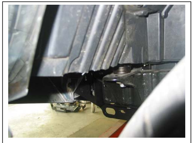
Figure 12: Trimmed under body guard, Passengers side shown
